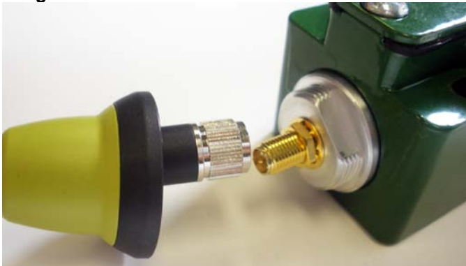
Figure 13. Limitless™ WGLA RP-SMA Connection, Integral
