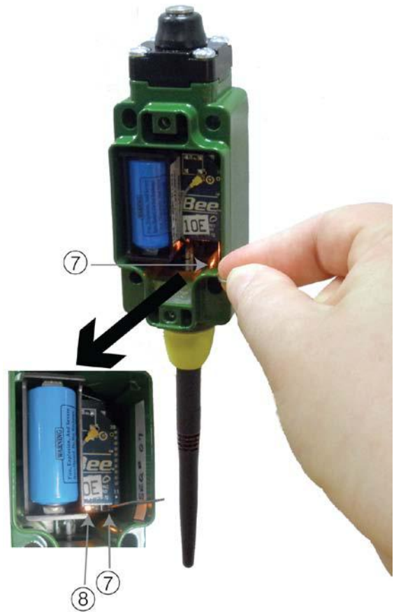
Figure 6. Limitless™ Switch with Function Button Depressed
