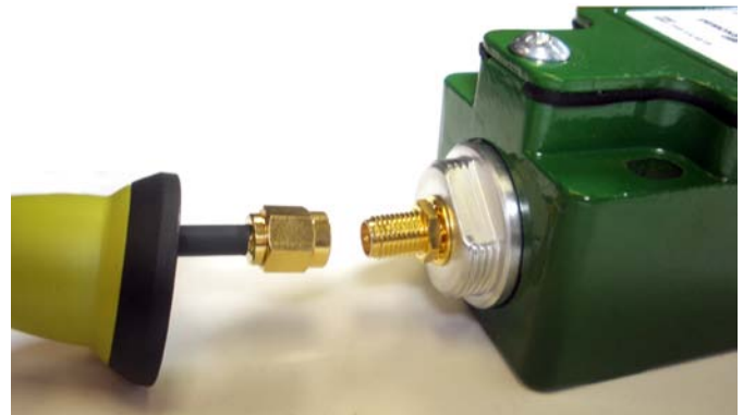
Figure 14. Limitless™ WGLA RP-SMA Connection, Remote
